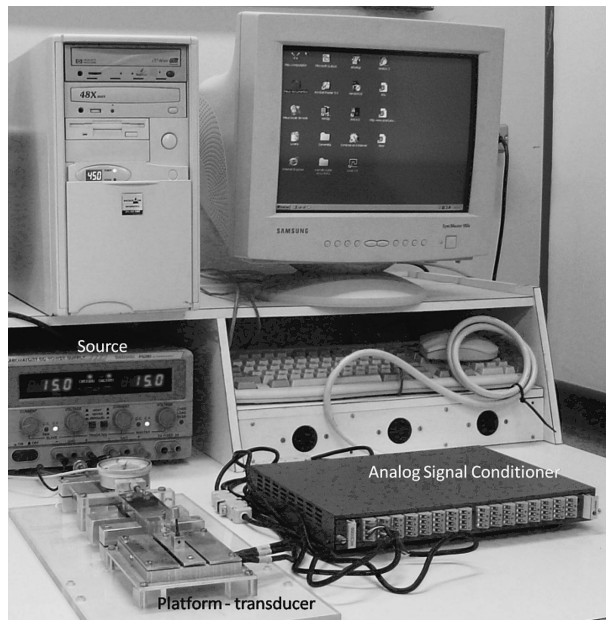
Figure 2 Transducer set. Platform (aluminum structure made up of a cross-shaped beam tied to its internal part, with 12 strain gauges; Power Source and Analogue Conditioner Signal Module).
